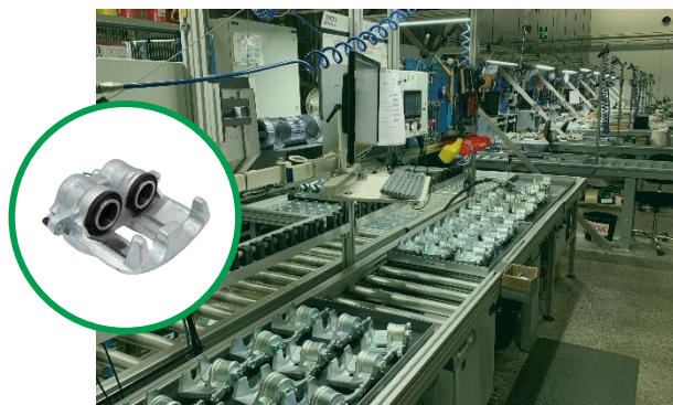
Automatic shuttle line Main production line
